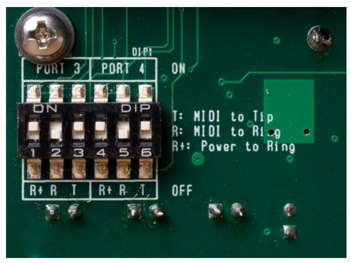
The first three switches on the left affect Port 3 while the three switches on the right affect Port 4.
