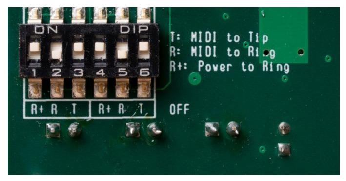
The first three switches on the left affect Port 3 while the three switches on the right affect Port 4.
