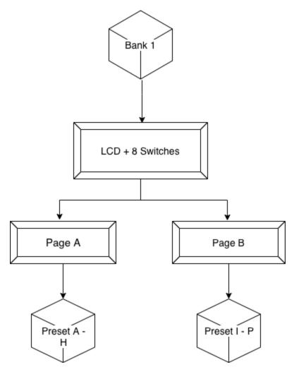
Each bank can display up to 8 presets, of which all are accessible from the 8 switches. The other 8 presets can be engaged via dual switch presses or external aux controllers. A Page Toggle function is also available via Switch B+C to switch between the first 8 presets and the last 8 presets.
