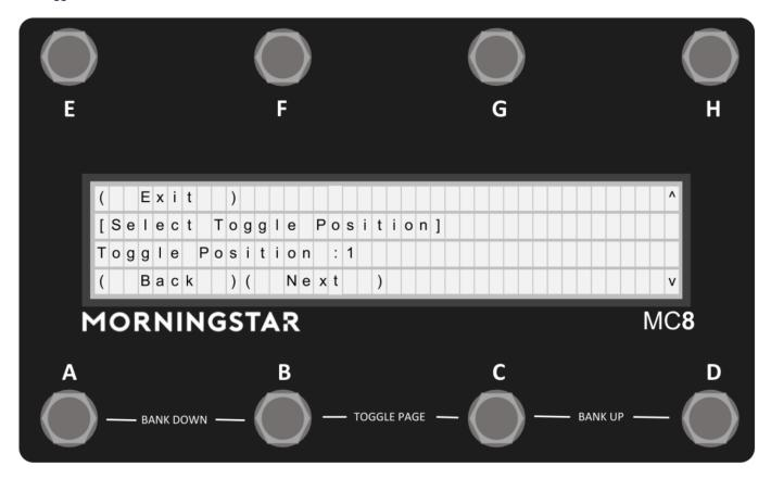
The next menu allows you to edit the message toggle position. Select between 1, 2 and Both. This allows only the messages that match the current preset toggle position to be invoked.
