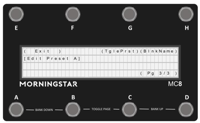
(TglePrst) - Toggles between On and Off for the preset toggle setting. If On, each time the preset is engaged, the toggle position of the preset will change. The Midi Messages in the preset will rely on the toggle position of the preset to determine if it should be invoked.
