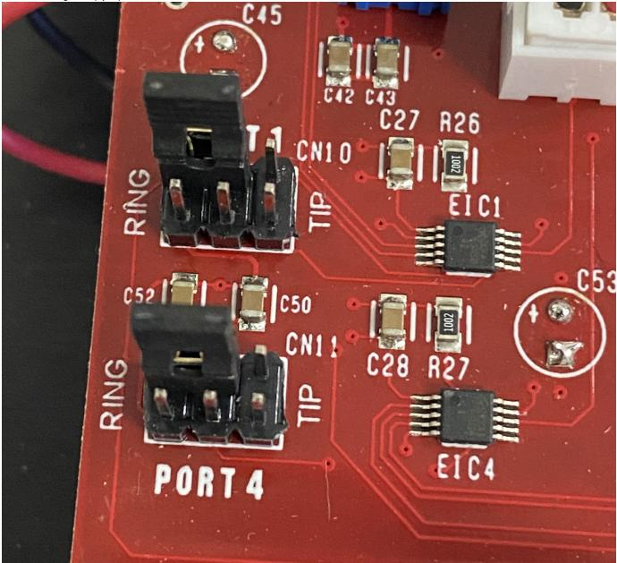
In the image above, Port 1 and Port 4 are configured to send MIDI to Chase Bliss devices.
