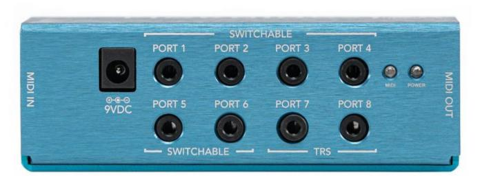
9VDC - Power the MIDI Box with a standard 9v DC centre-negative power supply with a minimum current draw of 20mA.
