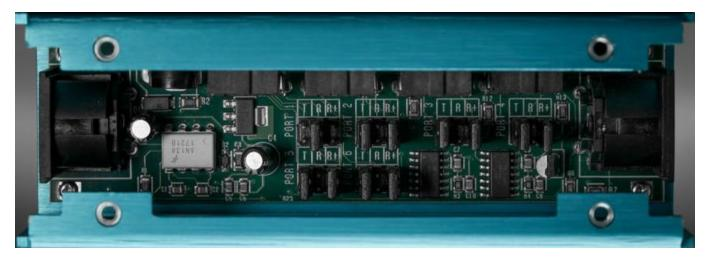
The internal jumper switches allow you to configure each port 1 to 6 to send MIDI via the tip or ring. You can also choose to have the ring powered or floating as some MIDI devices require. This makes the MIDI Box compatible with any MIDI TRS MIDI device.
