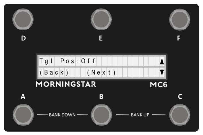
The next menu allows you to edit the message toggle position. Select between On and Off. This allows only the messages that match the current preset toggle position to be invoked.
