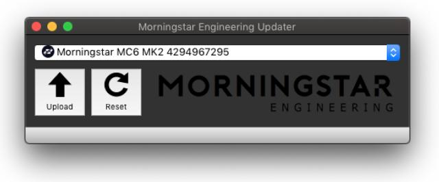
If your device is connected, it will appear in the Firmware Uploader software.
